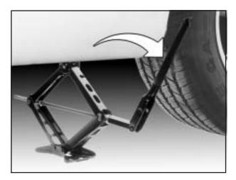
Raise the vehicle by turning the jack handle clockwise. Raise the vehicle far enough off the ground for the compact spare tire to fit underneath the wheel well of the vehicle. 5. Remove all wheel nuts and take off the flat tire.
